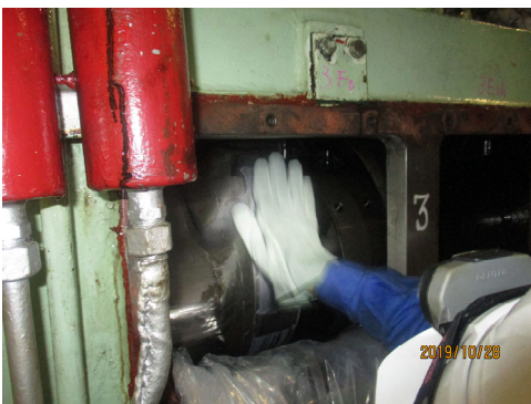
Rubbing in on the surface with leather glove
